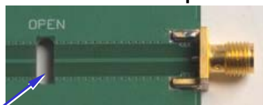
Hole minimizes stray capacitance
