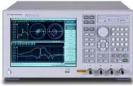
ENA self-contained RF balanced measurement solution for R&D or mfg
